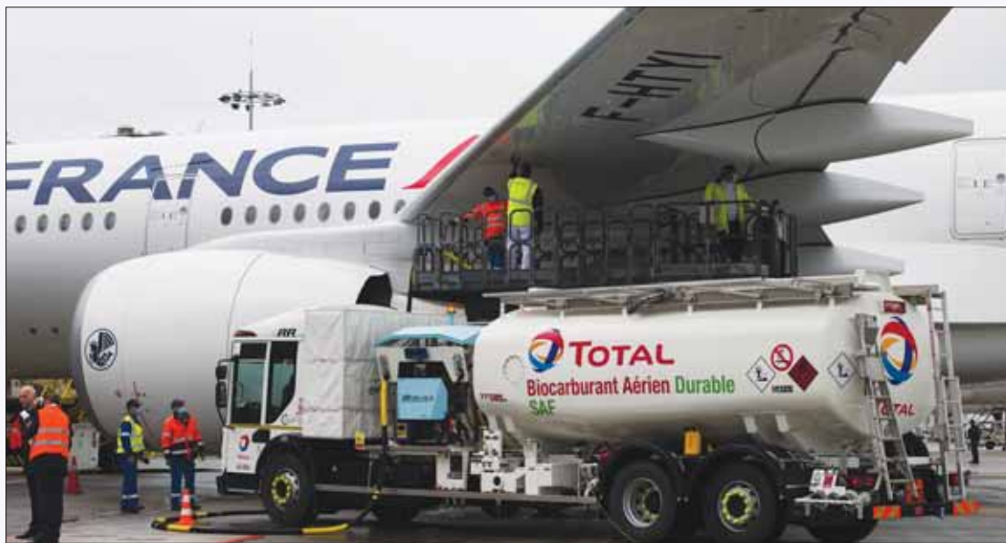
Workers connect a tanker truck filled with sustainable aviation fuel to a plane at Charles de Gaulle airport in Roissy, France. The use of SAF is rapidly advancing, with global production projected to nearly double this year as airlines around the world sign agreements with producers to purchase future SAF production.
