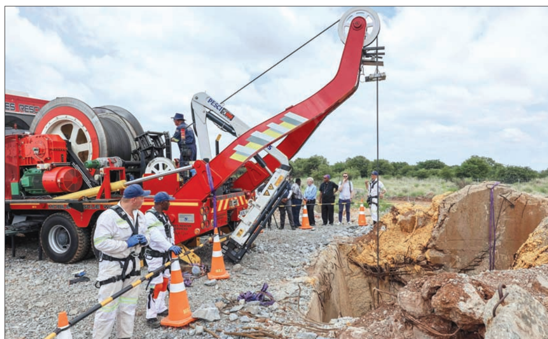
Metalliferous Mobile Rescue Winder operators look on as a cage is lifted from an abandoned gold shaft in Stilfontein.
